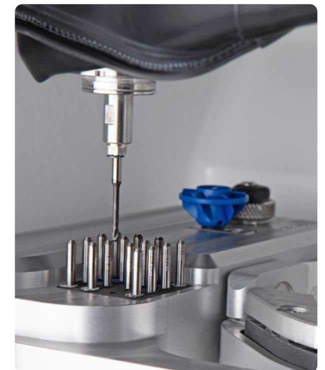
The automatic tool magazine with space for 16 standard tools plus an airtool .
