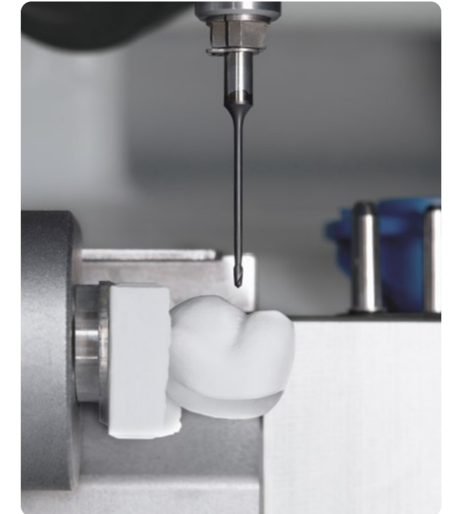
... and turn your talented E4 into a dry milling machine you can use to process materials such as zirconia, PMMA and various composites.
