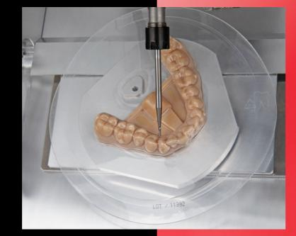
The tool-free clamping system further simplifies your work processes. This quick workpiece change enables you to produce entire series of aligners quickly and easily.
